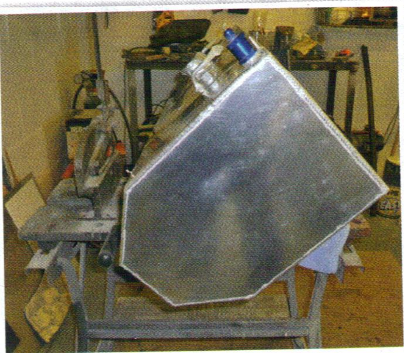
The new petrol tank, a little different to the one normally fitted to E-types!
